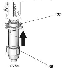
14. Hand tighten jam nut (122). Then tighten securely 1/8 to 1/4 turn with hammer or torque to 330 ft-lb (447.4 N•m).
