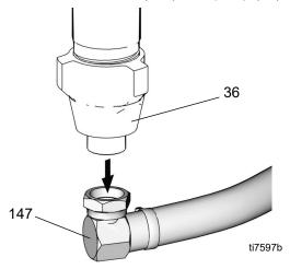
4. Remove paint and drain lines from filter housing.
